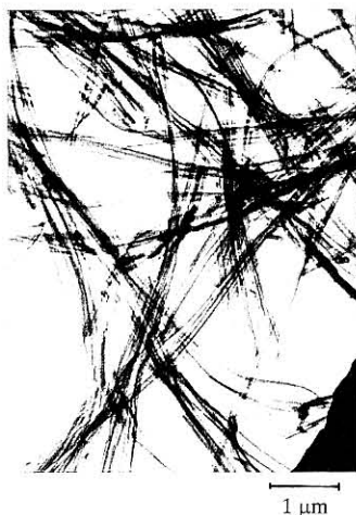
Figure 1. TEM image (15000 × magnification) for the reaction product of zinc hydroxide with benzoylchloride in acetonitrile.
